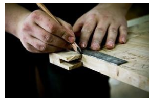
Measuring and marking out
