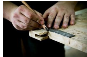
Measuring and marking out
